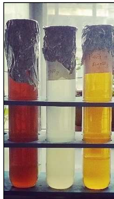
Fig.1. a).Banana extract treated with \text{AgNO}_3 b). \text{AgNO}_3 solution c). Orange extract treated with \text{AgNO}_3
